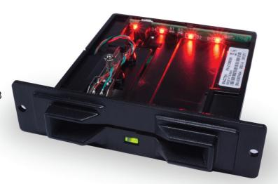
Optional always-on internal LED's offer slot illumination in low light environments. (PN:21066056)
